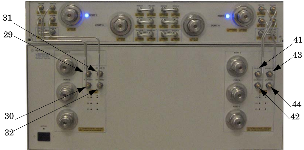
Figure 31 N5242A RF Interface Cable Connections
