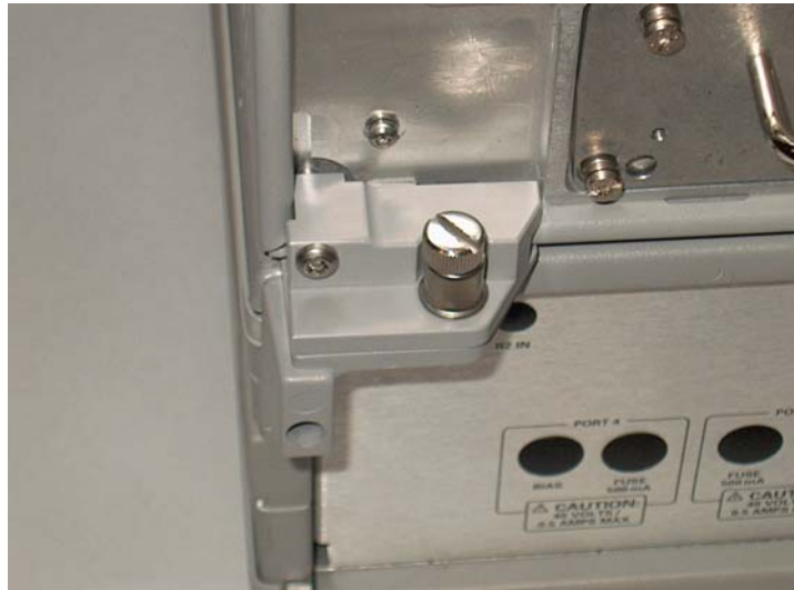
Figure 11 Locking Feet Screws
