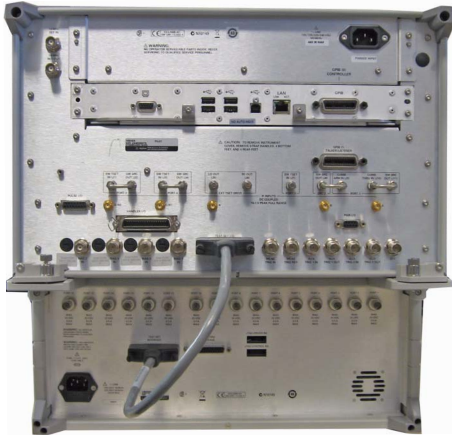
Figure 32 N5242A Test Set I/O Cable Connection
