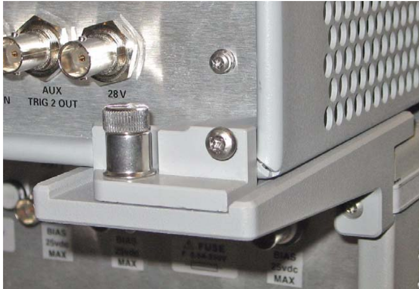
Figure 30 Locking Feet Screws
