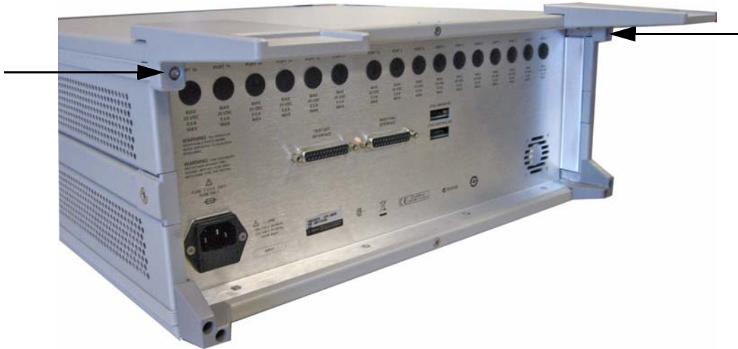
Figure 28 Install Locking Feet on U3022AM06
